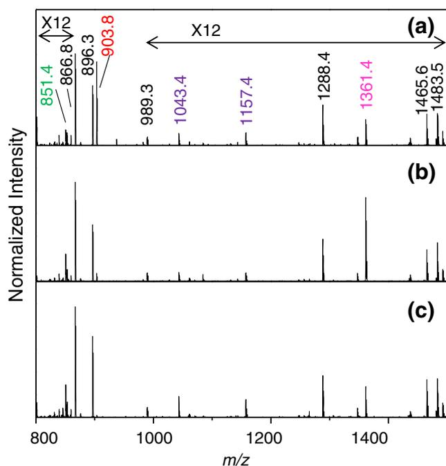
**Figure 4.** CID spectra of the mobility-selected ions at **(a)** 20.2, **(b)** 20.6, and **(c)** 21.0 ms. Unique fragments are labeled in colors (Figure 3) and nonspecific fragments are shown in black. The  $m/z$  range has been narrowed (800 to 1500) for a closer comparison between the spectra
