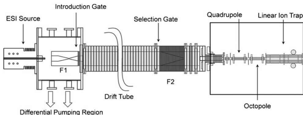
**Figure 1.** Schematic representation of the IMS-MS instrument used in these studies. The instrument is comprised of an ESI source, a drift tube, and a linear ion trap. See the section 2 for additional details
