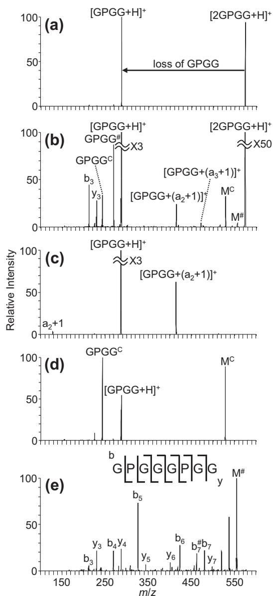
**Fig. 1.** Fragmentation spectra of  $[2\text{GPGG} + \text{H}]^+$  obtained by (a) CID and (b) 157 nm irradiation. The superscripted C and # indicate the losses of  $\text{CHO}_2$  and  $\text{H}_2\text{O}$ , respectively. CID spectra of (c)  $[\text{GPGG} + (\text{a}_2 + 1)]^+$ , (d) the  $\text{CHO}_2$ -loss product ( $\text{M}^\#$ ), and (e) the water-loss product ( $\text{M}^\#$ ) in spectrum b. The peaks in spectrum e are assigned according to the peptide sequence, GPGGGPGG.
