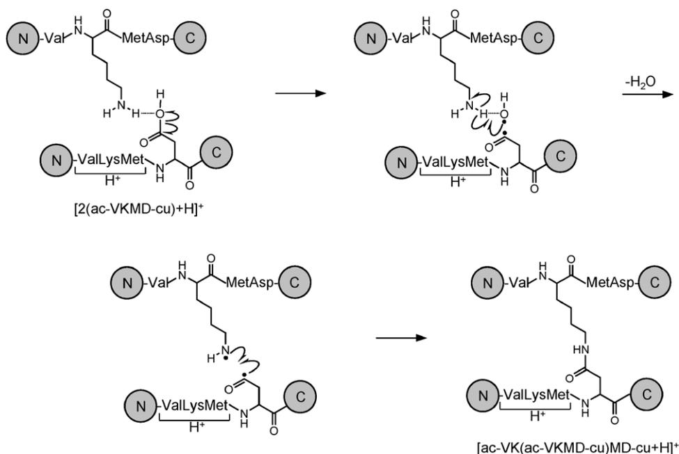
**Scheme 2.** Proposed mechanism for formation of a cross-linked peptide ion between Lys and Asp amino acid residues of separate peptide ions obtained from the [2(ac-VKMD-cu)+H]<sup>+</sup> complex upon 157 nm irradiation. The circled N and C at the end of each peptide indicate N- and C-termini blocking groups, respectively.
